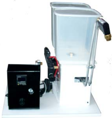
Air Drive w/ Shot Control & Mixer Manifold
